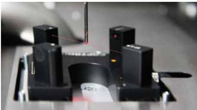
Needle measuring cross with auto-correction
